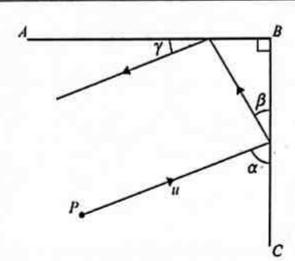
The smooth vertical walls AB and CB are at right angles to each other. A particle P is moving with speed u on a smooth horizontal floor and strikes the wall CB at an angle  $\alpha$ . It rebounds at an angle  $\beta$  to the wall CB. The particle then strikes the wall AB and rebounds at an angle  $\gamma$  to that wall (see diagram). The coefficient of restitution between each wall and P is e.
