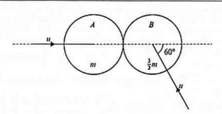
Two uniform smooth spheres A and B of equal radii have masses m and  $\frac{3}{2}m$  respectively. The two spheres are each moving with speed u on a horizontal surface when they collide. Immediately before the collision A's direction of motion is along the line of centres, and B's direction of motion makes an angle of 60° with the line of centres (see diagram). The coefficient of restitution between the spheres is  $\frac{2}{3}$ .
