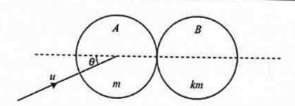
Two uniform smooth spheres A and B of equal radii have masses m and km respectively. Sphere A is moving with speed u on a smooth horizontal surface when it collides with sphere B which is at rest. Immediately before the collision, A's direction of motion makes an angle  $\theta$  with the line of centres (see diagram). The coefficient of restitution between the spheres is  $\frac{1}{3}$ .
