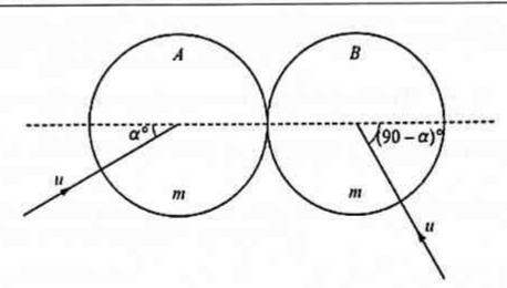
Two uniform smooth spheres A and B of equal radii each have mass m. The two spheres are each moving with speed u on a horizontal surface when they collide. Immediately before the collision A's direction of motion makes an angle of  $\alpha^{\circ}$  with the line of centres, and B's direction of motion is perpendicular to that of A (see diagram). The coefficient of restitution between the spheres is e.
