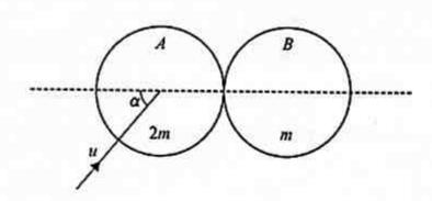
Two uniform smooth spheres A and B of equal radii have masses 2m and m respectively. Sphere B is at rest on a smooth horizontal surface. Sphere A is moving on the surface with speed u and collides with B. Immediately before the collision, the direction of motion of A makes an angle  $\alpha$  with the line of centres of the spheres, where  $\tan \alpha = \frac{4}{3}$  (see diagram). The coefficient of restitution between the spheres is  $\frac{1}{3}$ .
