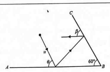
AB and BC are two fixed smooth vertical barriers on a smooth horizontal surface, with angle  $ABC = 60^{\circ}$ . A particle of mass m is moving with speed u on the surface. The particle strikes AB at an angle  $\theta$  with AB. It then strikes BC and rebounds at an angle  $\beta$  with BC (see diagram). The coefficient of restitution between the particle and each barrier is e and  $\tan \theta = 2$ .
