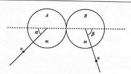
Two uniform smooth spheres A and B of equal radii each have mass m. The two spheres are each moving with speed u on a horizontal surface when they collide. Immediately before the collision, A's direction of motion makes an angle  $\alpha$  with the line of centres, and B's direction of motion makes an angle  $\beta$  with the line of centres (see diagram). The coefficient of restitution between the spheres is  $\frac{1}{3}$  and  $2\cos\beta = \cos\alpha$ .
