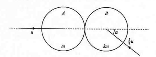
Two uniform smooth spheres A and B of equal radii have masses m and km respectively. The spheres are moving on a horizontal surface with speeds u and  $\frac{5}{8}u$  respectively. Immediately before the spheres collide, A is travelling along the line of centres, and B's direction of motion makes an angle  $\alpha$ with the line of centres (see diagram). The coefficient of restitution between the spheres is  $\frac{2}{3}$  and  $\tan \alpha = \frac{3}{4}$ .
